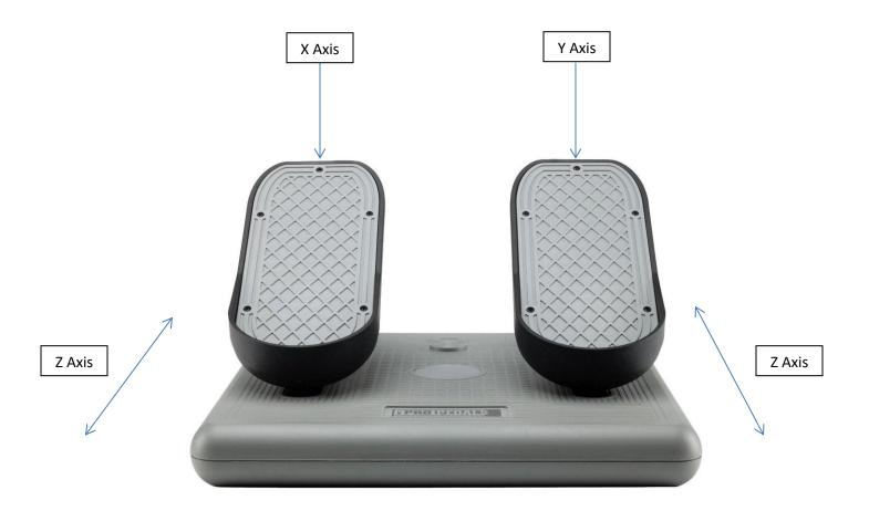
X Axis = Pushing Left Pedal. In FS2020, assign "Left Brake Axis" to "Joystick L-Axis X" Y Axis = Pushing Right Pedal. In FS2020, assign "Right Brake Axis" to "Joystick L-Axis Y" Z Axis = Sliding motion back and forth. In FS2020, assign "Rudder Axis" to "Joystick L-Axis Z"
